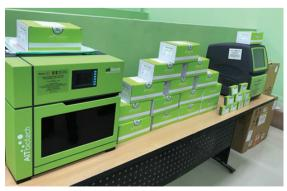
[Real-Time PCR machine, Nucleic Acid Extraction machine, PCR detection kits and DNA & RNA extraction kits]
